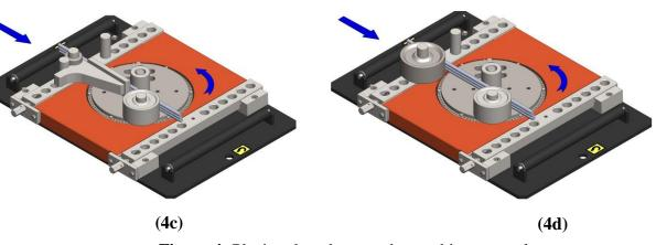
Figure 4: Placing the rebars on the machine correctly
