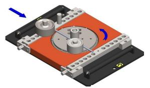
Fixing the rebars to be b (4b) he machine in multi-rebar bending with the help of bending sleeves. (4d)
