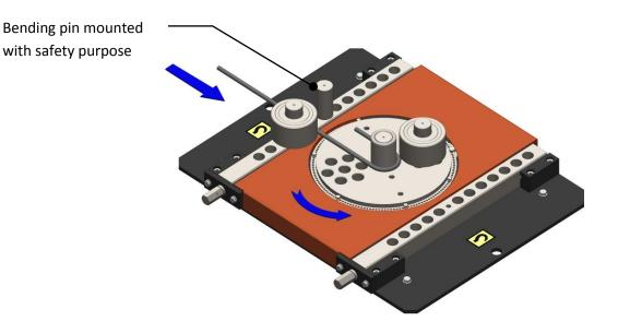
Figure12: Hook Bending demo
