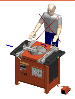
Figure 7: Wrong positioning of the person making bend
