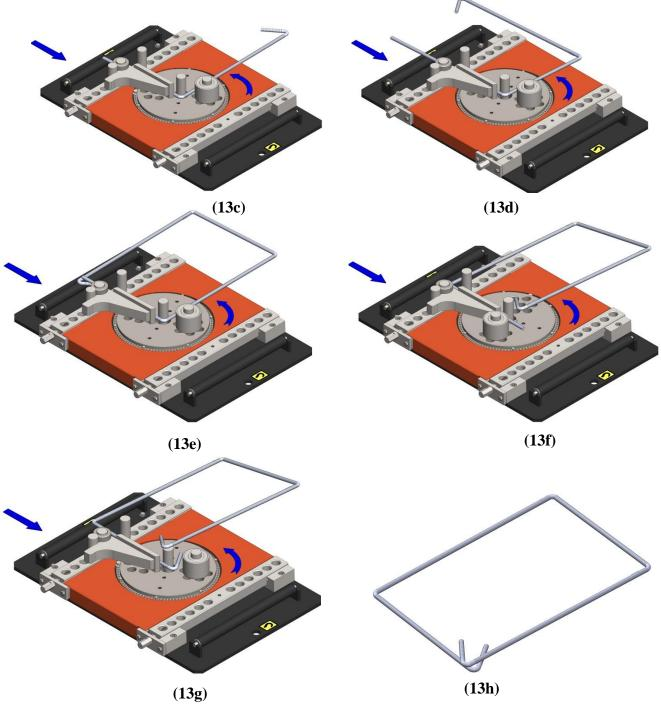
Figure13: Stirrup bending demonstration
