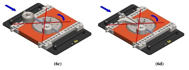
Figure 6: Wrong placement of the rebars on the machine
