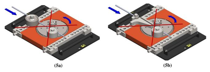
Figure 5: Incorrect placement of the rebars on the machine
