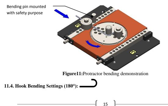
It is set with the same method carried out in bent bar bending by pressing the P3 button on the control panel.
